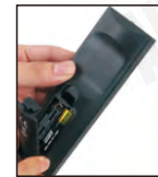
Insert the new battery into the battery holder with the + side facing upwards.
