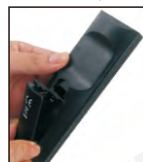
Pull out the battery holder and remove the old battery.
